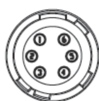
(B) Power/I/O Signal Connector Hirose HR10A-7R-6PB equivalent Depending on the camera settings, trigger signal input can be performed.
